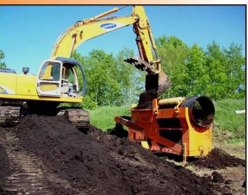
While Paso Robles keeps its EZ-Screen 409 Trommel Screener in their yard, the machine is designed to be trucked to and from different job sites. Set up is quick, and once ready for action, the EZ-409 works well paired with 1/4-yard to 2-yard loaders.
